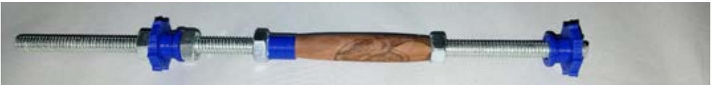
Choosing your pulley is simple. Match up the blank to the pulley that is closest to its outside diameter. Once you've chosen a pulley set up the axle like the picture above. From left to right: Nut, Rotor, Nut, Nut, Pulley, Turning Bushing, Blank, Turning Bushing, Nut, Rotor. Note that if you're a blank with a 7mm tube the bushings are not needed.
